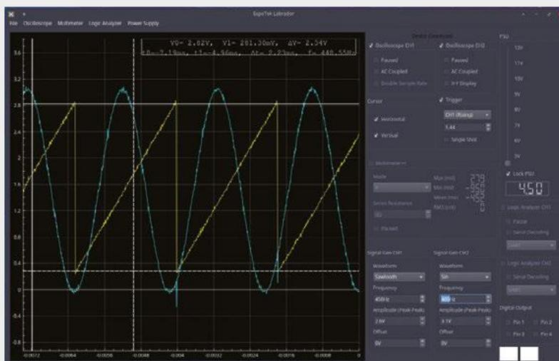
settings and configuration options to the most useful and common. However, it's also capable of some serious circuit and microcontroller analytics; various trigger values can be used to synchronise waveforms, serial messages can be decoded in real time from the logic analyzer, and grabbed values can be saved as a CSV text file.
